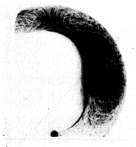
FIG. 13. Steady flow pattern for low Rayleigh numbers with 350 cS silicone fluid.
